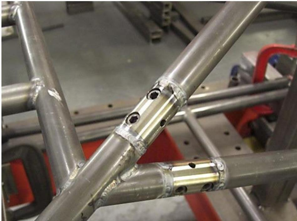
Both engine side spars are also removable, utilising the same clevis joint arrangement for optimal strength and function. This construction, in combination with 'Veed' engine mounting plates, affords quick and easy removal of the entire engine with the minimal disassembly of ancillaries.
