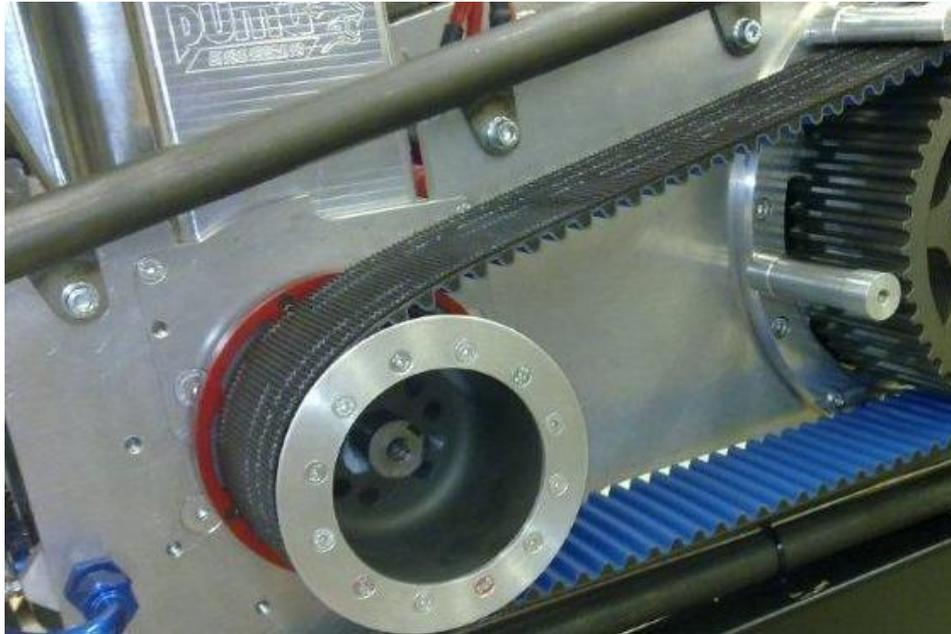
Although 'Veed' plates are not new, they are usually left open but Puma have improved on the design by designing removable sections that will afford the same level of strength in the plates as those without cut out 'Veeds'.
