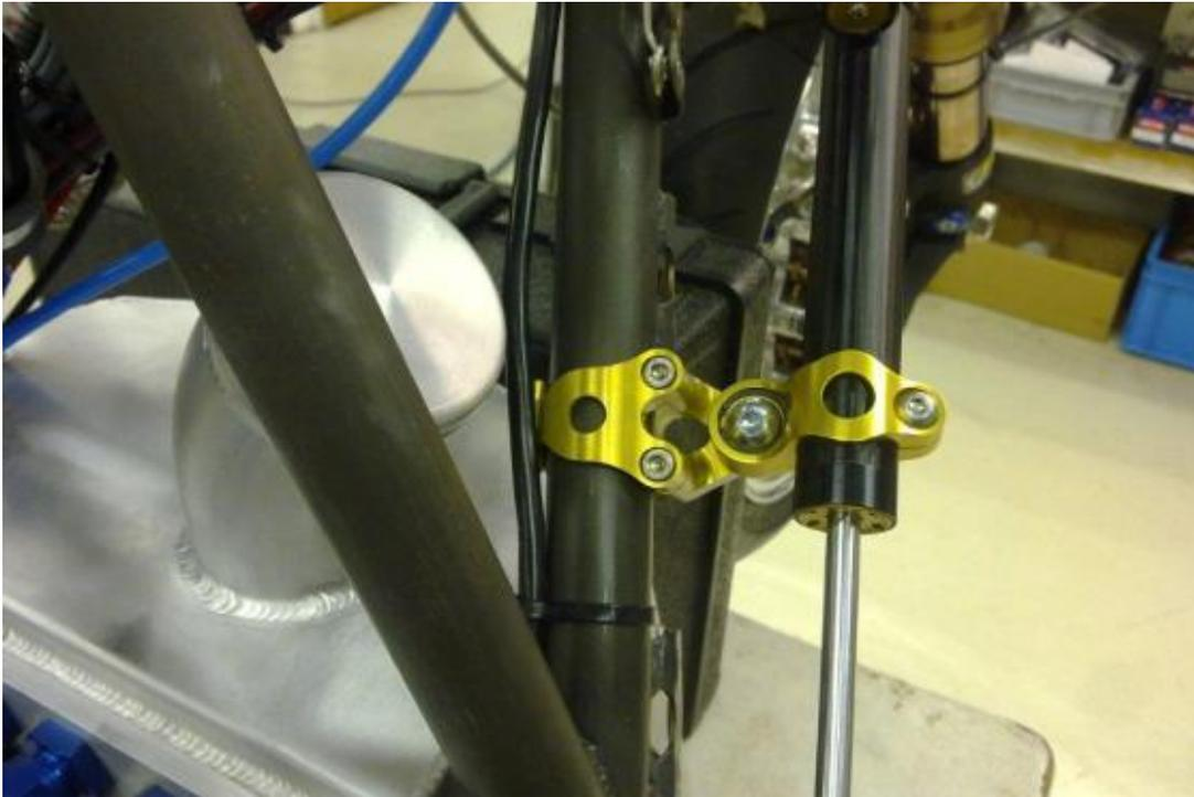
Front suspension and steering damping are courtesy of [Hyperpro](#), the leading supplier of progressive suspension units for motorcycles. They took the standard Showa forks and reworked them with springs better suited to the dynamics of the bike characteristics, shortened, revalved and with heavier oil. A pair of 140mm stroke linear CSC units - fast becoming the damper of choice on high performance dragbikes in Europe - was chosen for steering damping.
